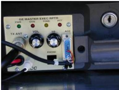
Discovered no discriminator audio present on the MCC accessory connector pin 11 (DB15). There was "Receiver Audio Output" on pin 2, but with de-emphasis filtering. We decided to use this connection but only until we could figure out why there was no discriminator audio at pin 11. The pin out of the DB15, as indicated on MCC's document is:
