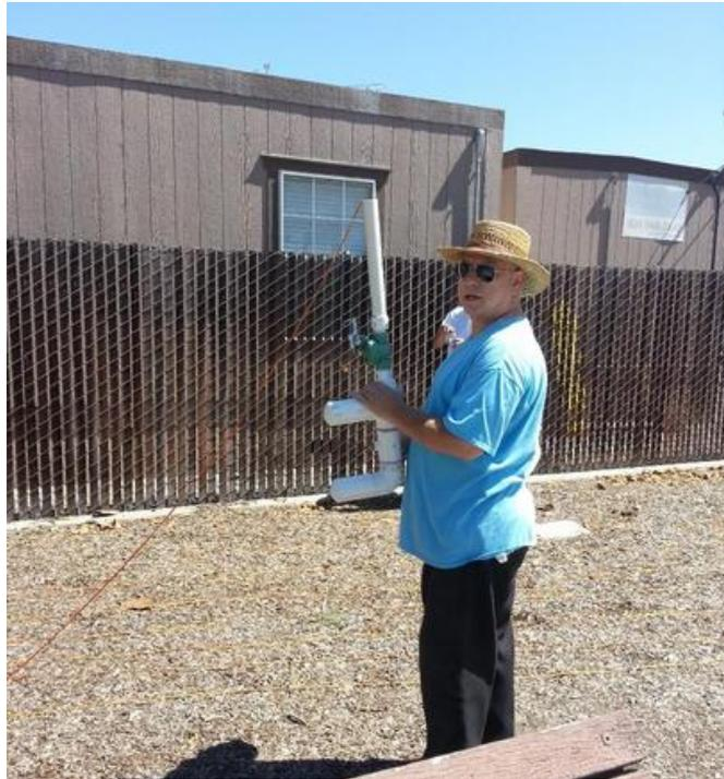
Jim Fahy (W6WKY) with his custom built rig to shoot up high a lead guide line for the antenna setup.
